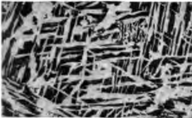
FIG. 5.—Gun steel, C. = 0.30%. From top of ingot as cast, magnified 29 diameters. Whites, ferrite; blacks, carbide.
