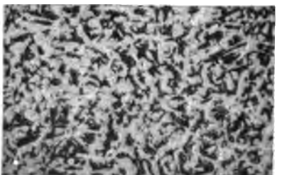
FIG. 6.—Gun steel, C. = 0.30%. From bottom of ingot as cast, magnified 29 diameters. Whites, ferrite; blacks, carbide.
