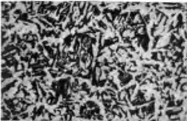
FIG. 7.—Gun steel, C. = 0.30%. Top of ingot, forged and annealed, magnified 29 diameters. Whites, ferrite; blacks, carbide.
